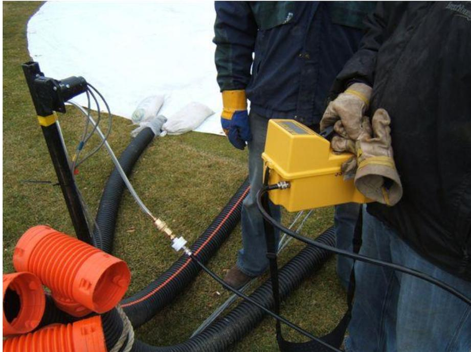
Picture of meter that collected and analyzed oxygen and carbon dioxide.
