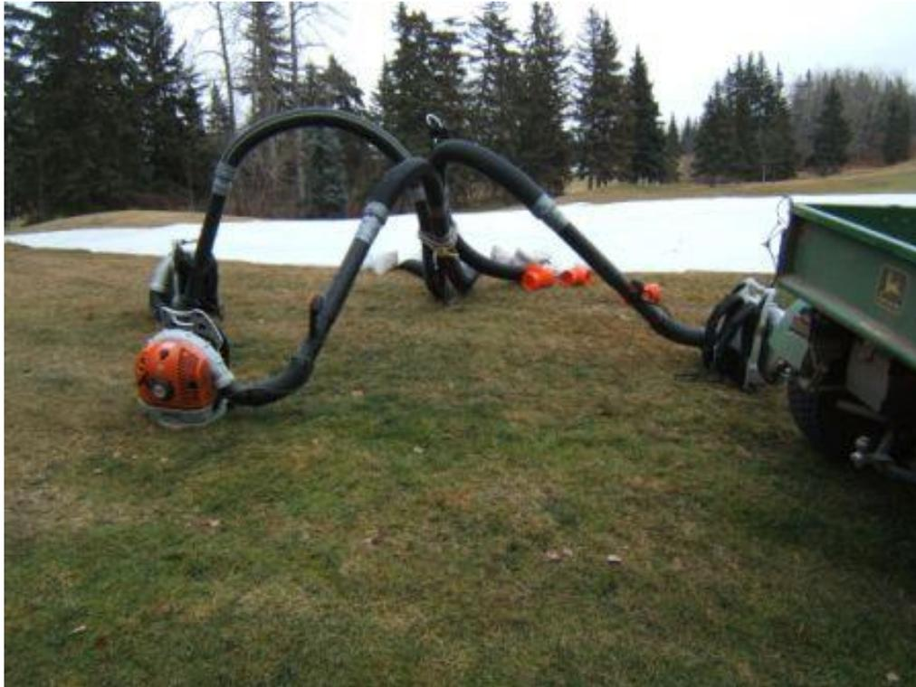
Picture shows leaf blowers attached to ventilation pipes.
