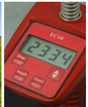
Figure 7: a) (left) Jenquip EC-10 for pasture biomass estimation; b) (right) Display showing available biomass (dry matter basis).
