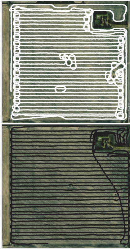
Figure 8. Top image shows autonomous spreading operation in 2023; bottom image shows a conventional self-propelled spreader operation in 2022.
