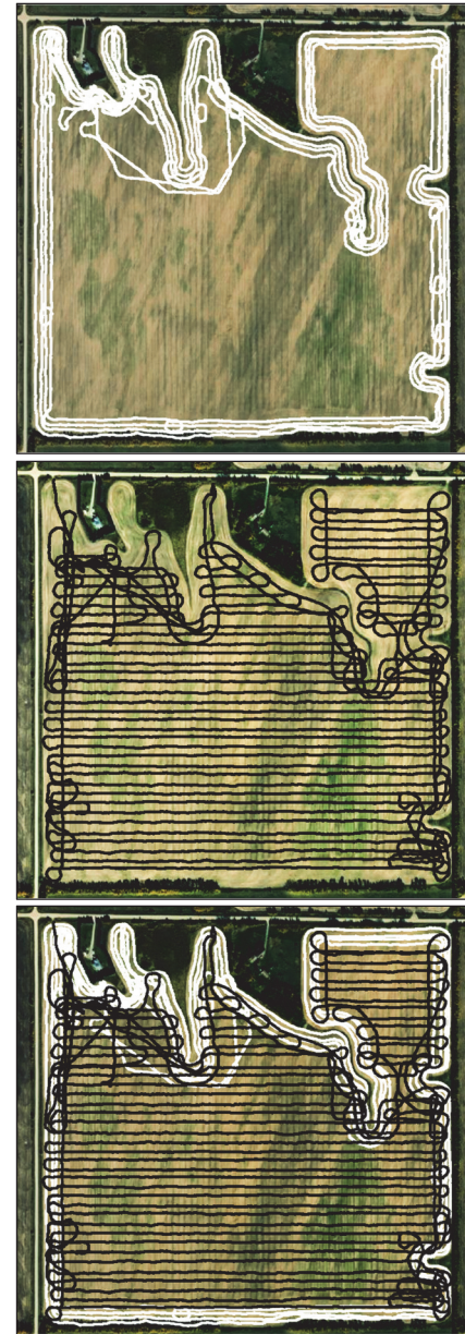
Figure 9. Synchronous seeding operation in central Alberta on May 23, 2022. Top image shows the white path of OP seeding the headlands, the middle image shows the path of a 2020 Case IH Steiger 420 with 2019 Seed Master Ultra SR seeding AB lines, and the bottom image shows the paths of both pieces of equipment as they worked simultaneously.
